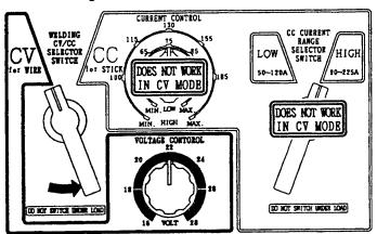
Figure 10. Welding Voltage Adjustment
